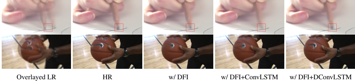
Figure 7: Ablation study on Deformable ConvLSTM (DConvLSTM). ConvLSTM will fail when meeting videos with fast motions. Embedded with state updating cells, the proposed DConvLSTM is more capable of leveraging global temporal contexts for reconstructing more accurate visual content even for fast motion videos.
